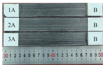
图14 连续纤维3D打印平板样件 Fig.14 Flat panel of continuous-fiber 3D printing
